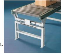
**CAPACITIES:** 300 Kg per frame. Total scale capacity is double the individual frame rating. When selecting a capacity, the weight of the conveyor section must be factored in.
